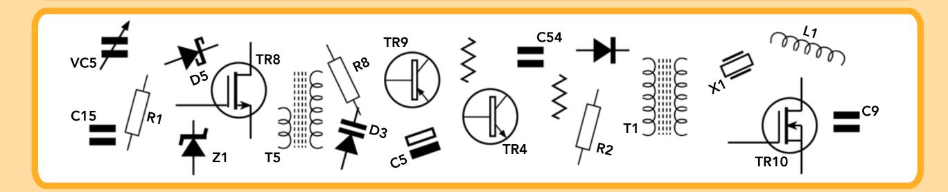
In order to standardise the way in which components are identified within schematics, the IEEE introduced a standard IEEE 200-1975 as the "Standard Reference Designations for Electrical and Electronics Parts and Equipments." This was later withdrawn and later the ASME (American Society of Mechanical Engineers), initiated the new standard ASME Y14.44-2008.
